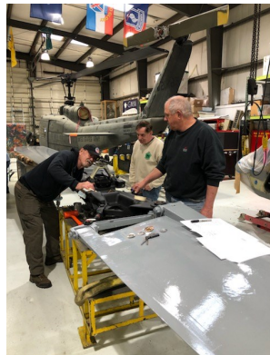
Mechanics inspecting rotor blades
