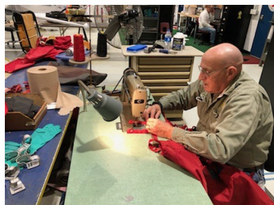
Fabricating new safety covers
